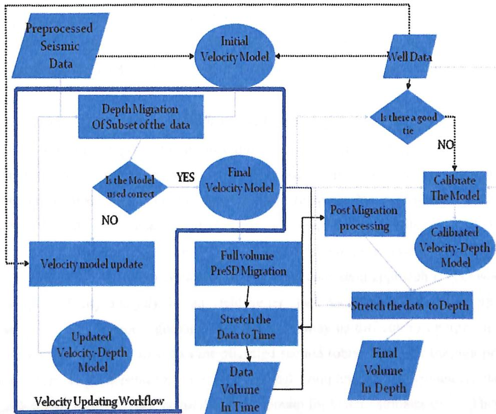
Figure 6: Generalized PSDM work flow
