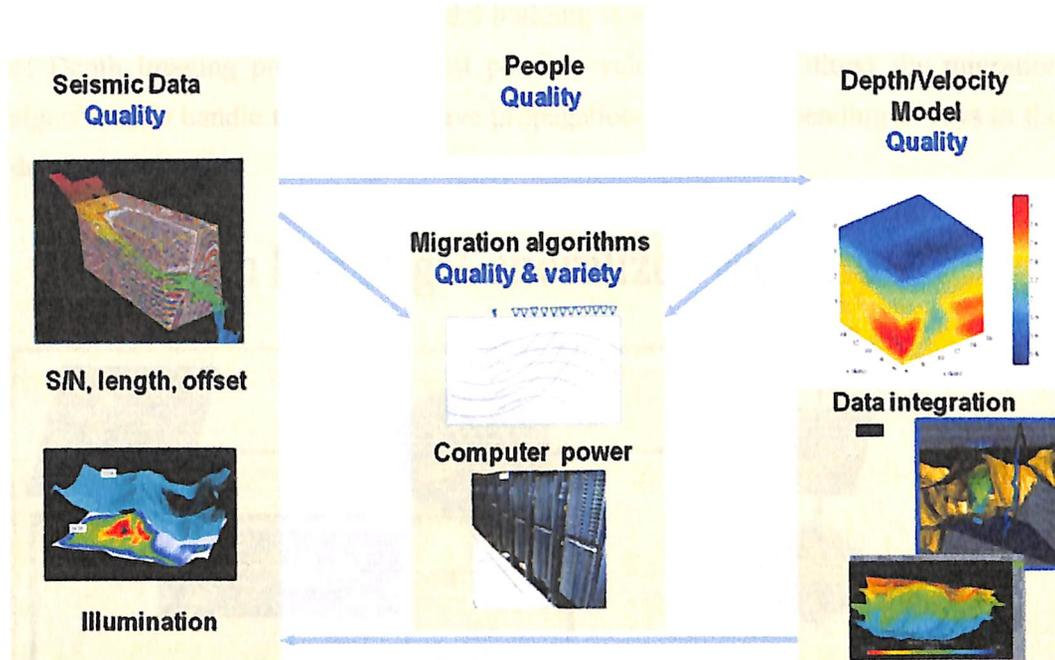
Figure 5: Inputs required for depth imaging
