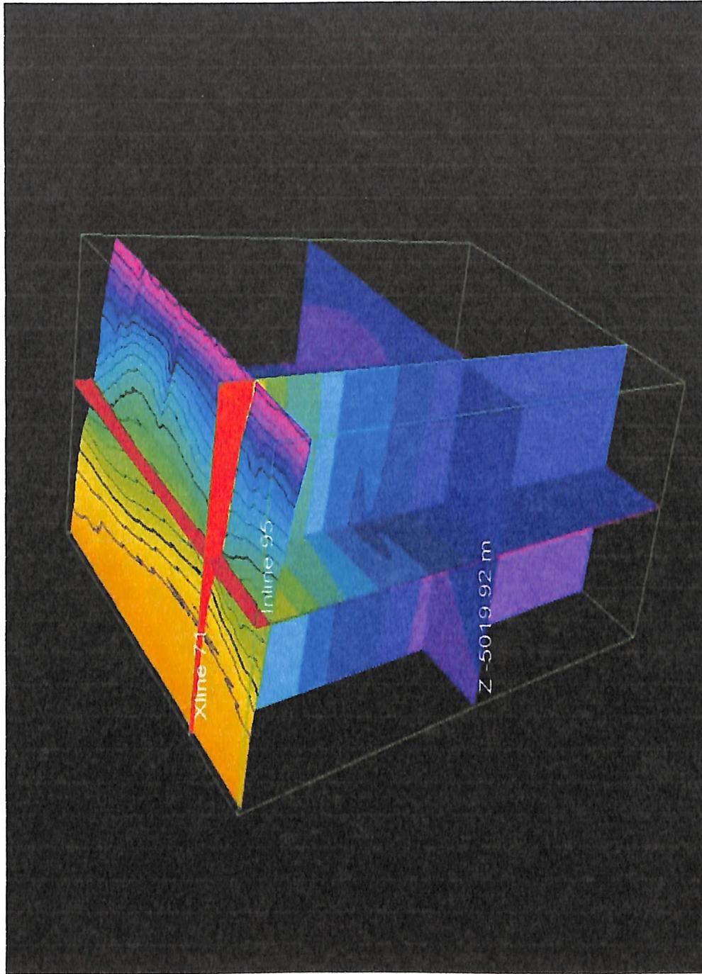
Plate 2: Initial velocity model with water bottom surface
