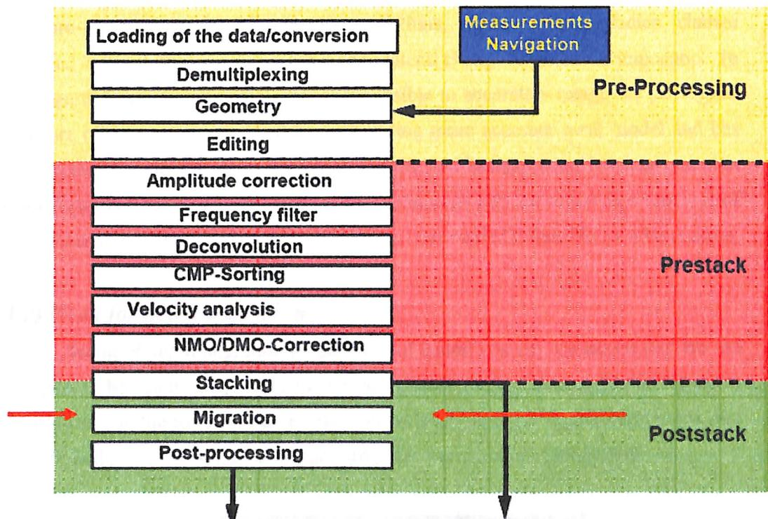
Figure 2 : Basic seismic data processing flow
