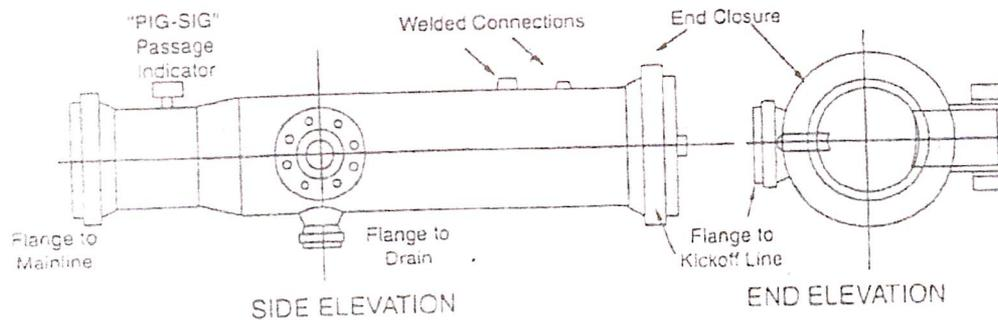
Figure 4-11: typical pig receiver
