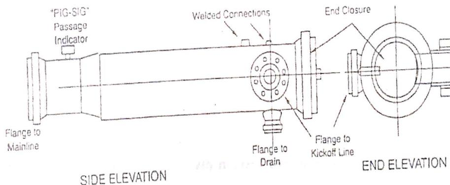
Figure 4.10: Typical Pig Launcher
