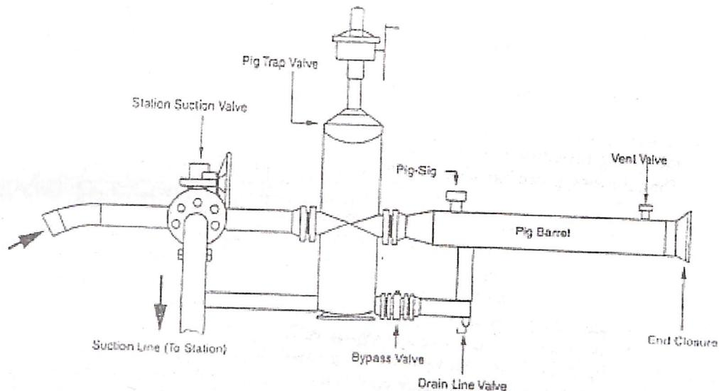
Figure 4.15: Typical pig receiver for liquid lines
