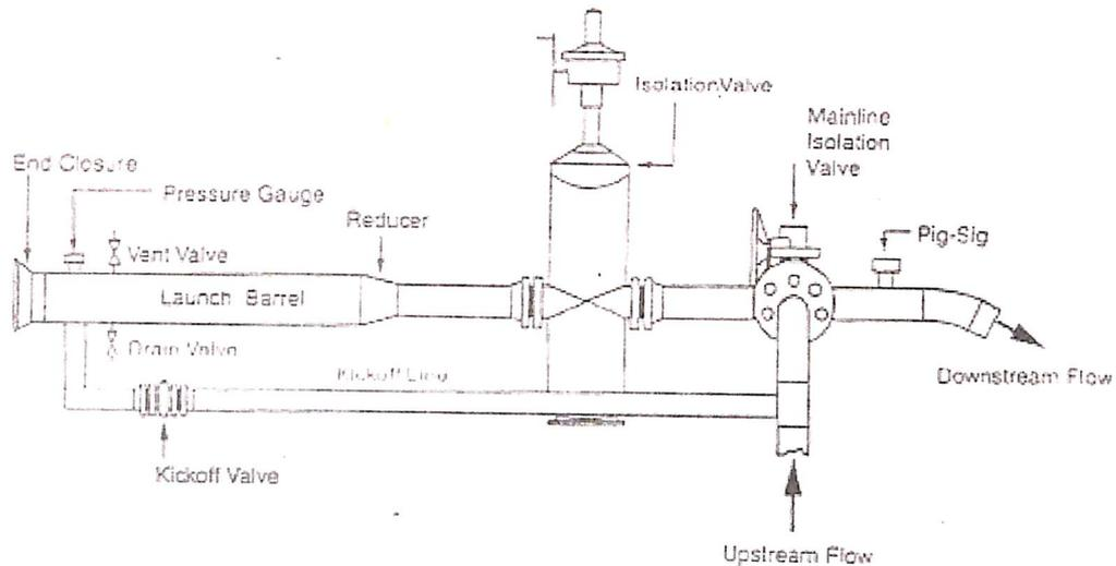
Figure 4-13: Typical Liquid line launching trap
