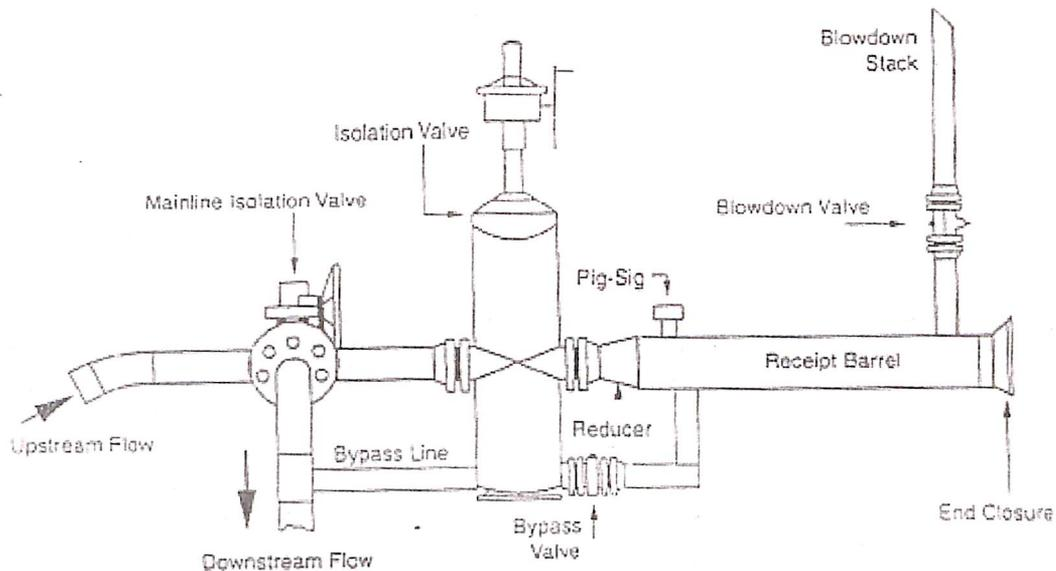
Figure 4.14: Typical pig receiver for gas lines
