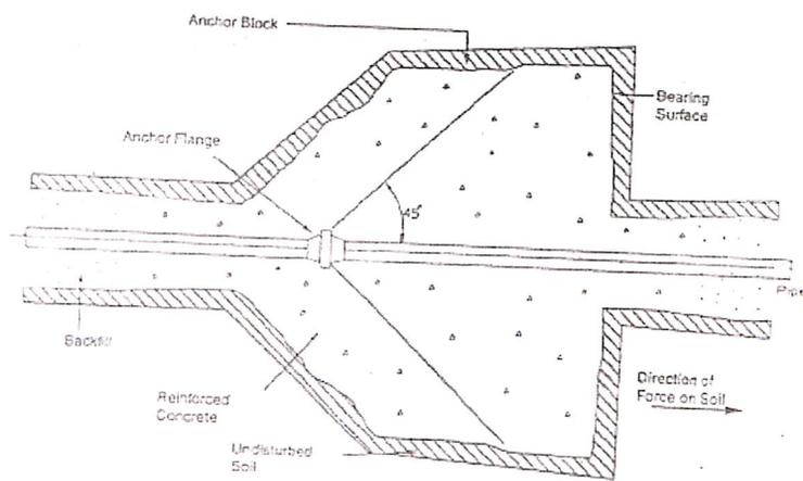
Figure 4-4 Plan view of anchor block
