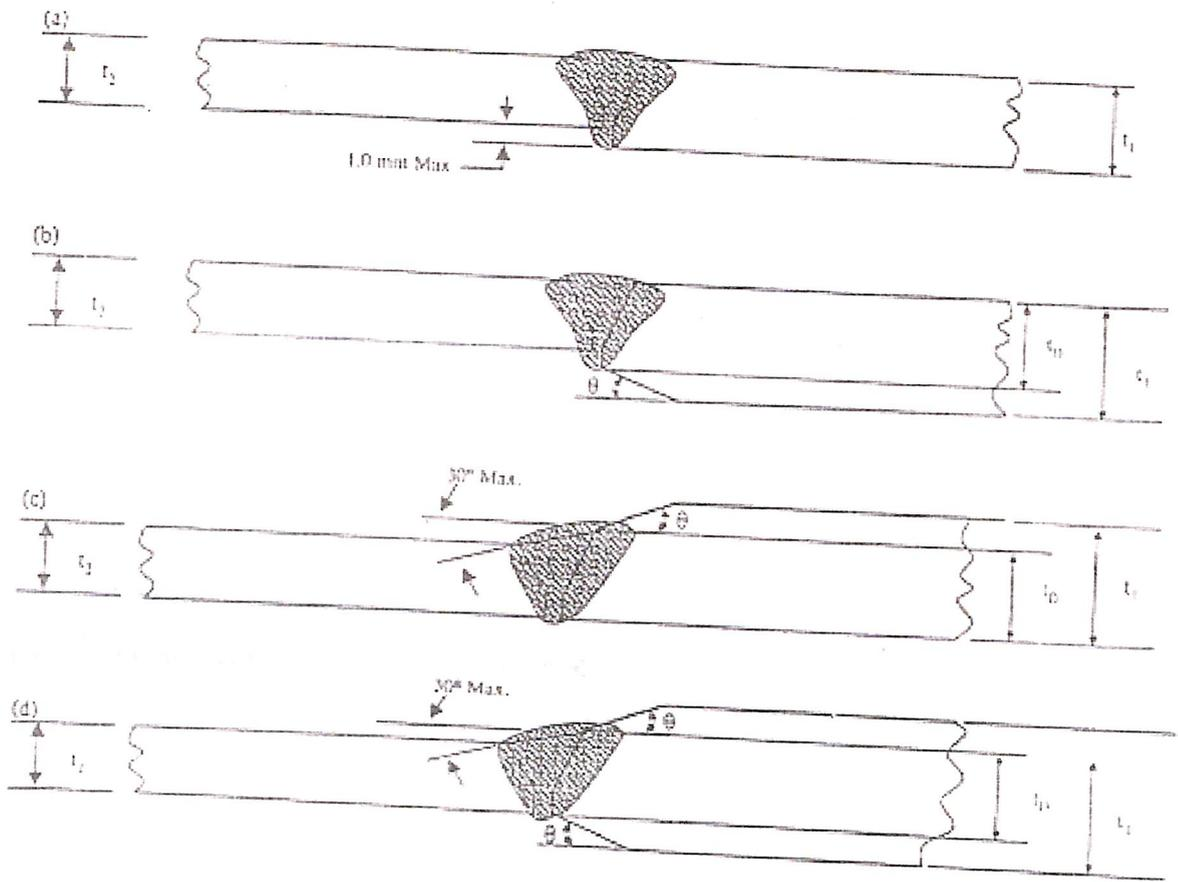
Figure 4.6: Back beveled joint design for piping design to operate at a hoop stress of 60% SMYS or less
