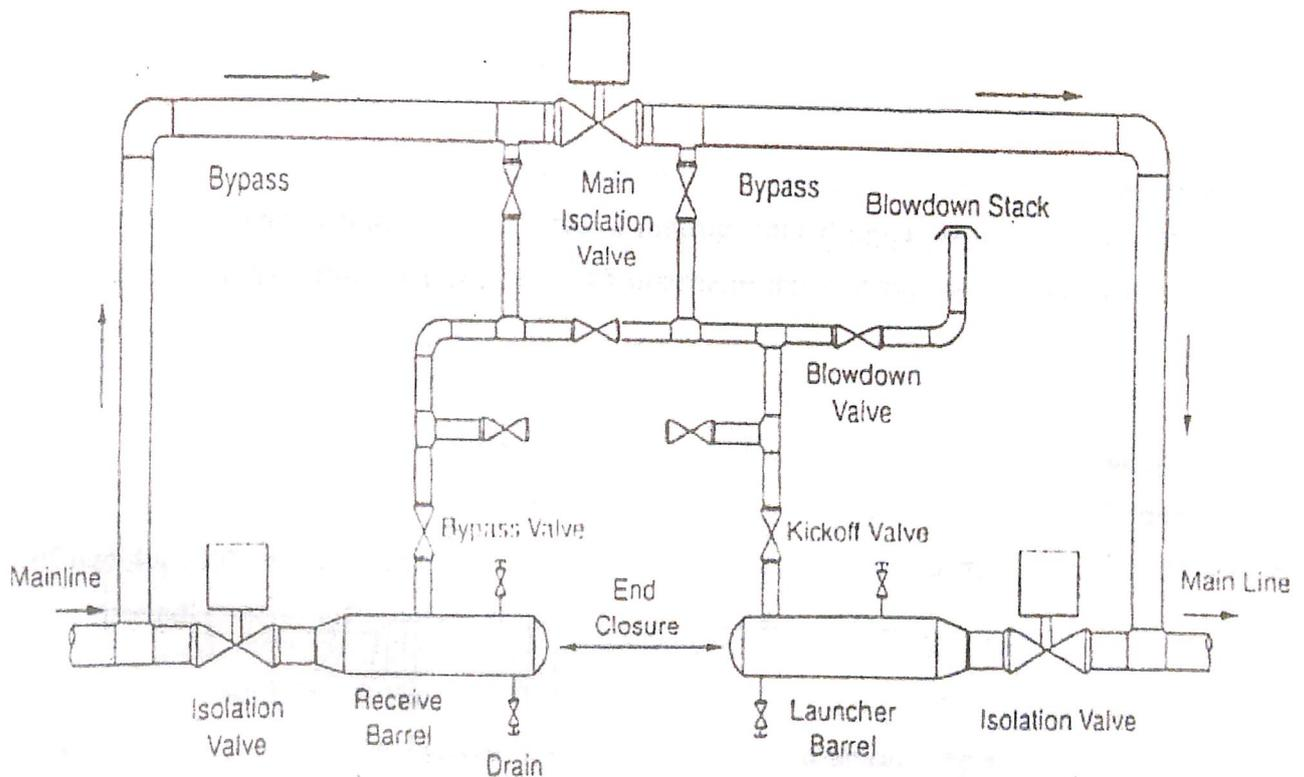
Figure 4.9: Scraper launcher/ Receiver
