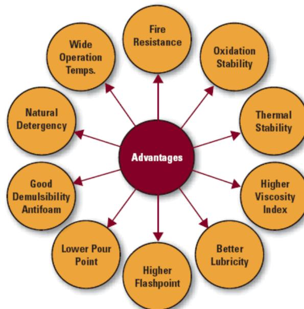
**Figure 2.8:** Operational advantages of synthetic oils
