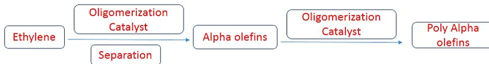
Figure 1.1 Conventional process for PAO synthesis
