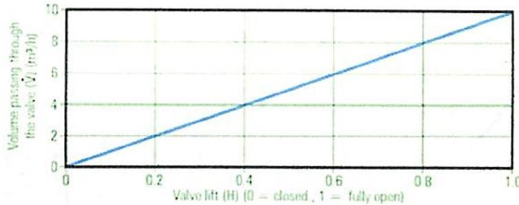
Fig. 7.2 Flow / lift curve for a linear valve
