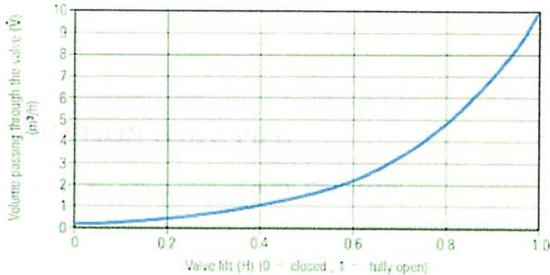
Fig. 7.3: Flowrate and valve lift for an equal percentage characteristic
