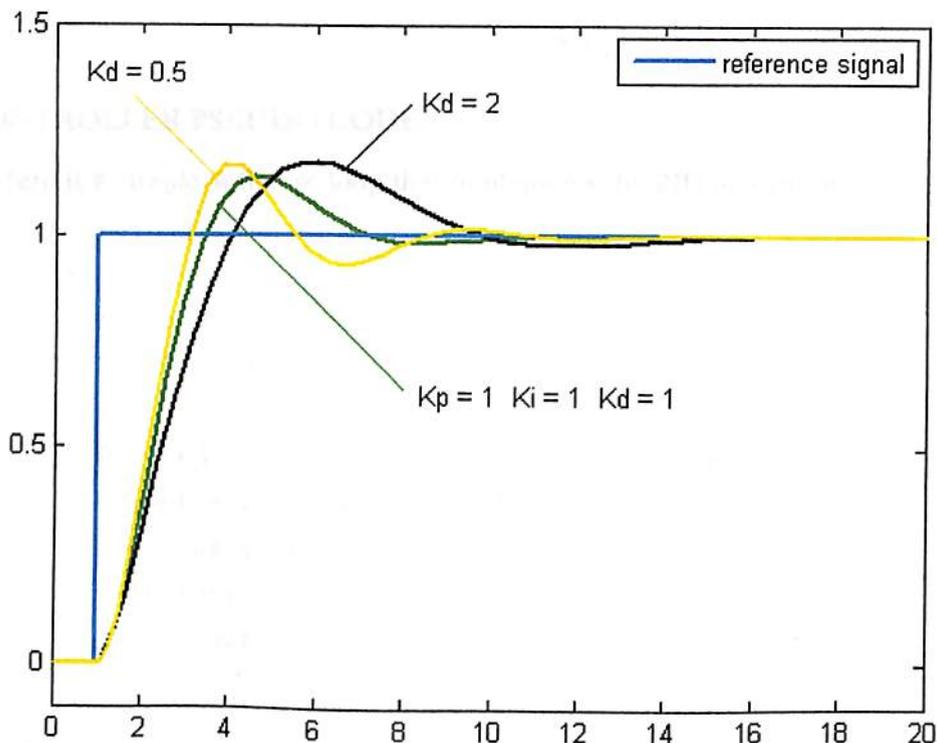
Fig. 4.7: Change of response for varying  $K_d$
