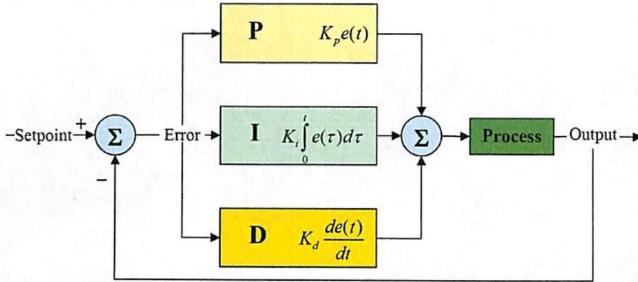
Fig. 4.3: A block diagram of a PID controller
