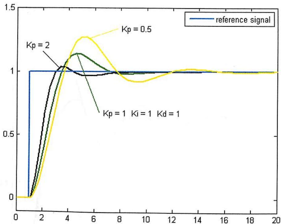
Fig. 4.5: Change of response for varying  $K_p$ .
