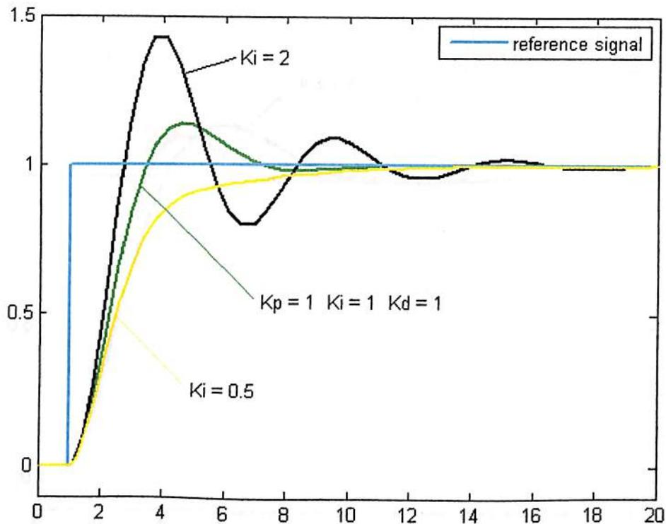
Fig. 4.6: Change of response for varying  $K$
