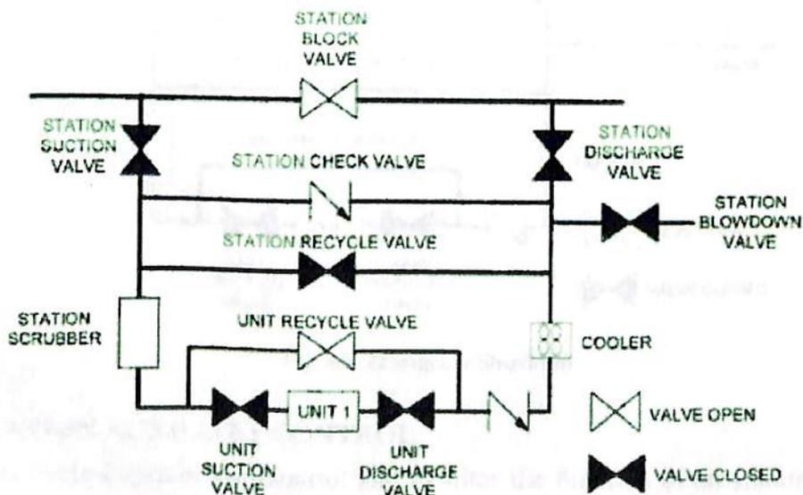
Fig. 3.2: Station Shutdown Lockout
