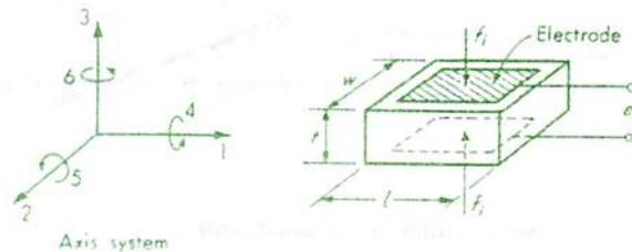
Fig.7.4 Piezoelectric Transducer.
