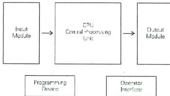
Fig. 5.2: Main Component of PLC
