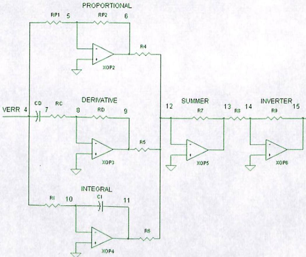
Fig. 4.4: Architectural diagram of a PID controller
