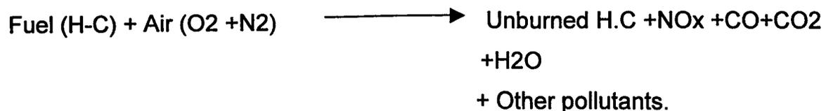
**2.1:: Emissions from a typical automobile / I.C Engines can be classified according to the source of emission:**
