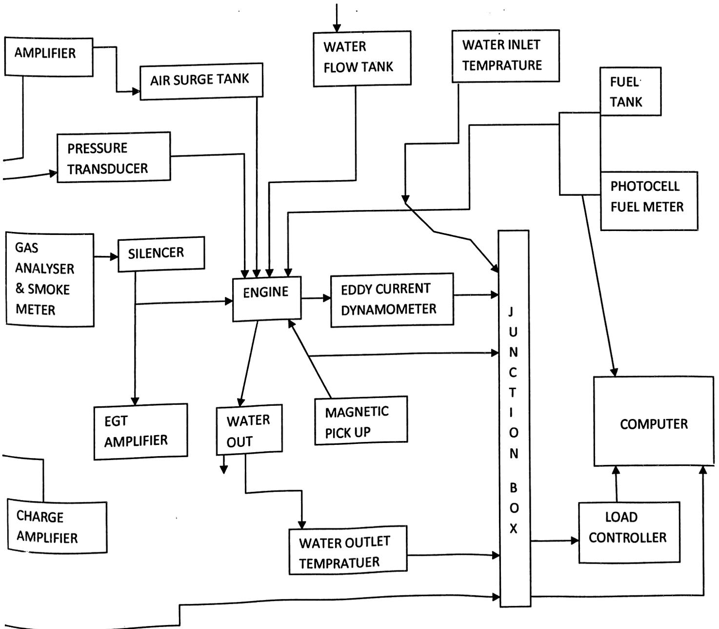
**4.1.1 Engine:** Engine used in the experiment is a 4 stroke cycled engine made by kirloskar oil engine limited. in a water cooled, naturally aspirated, direct injection engine having specifications:-
