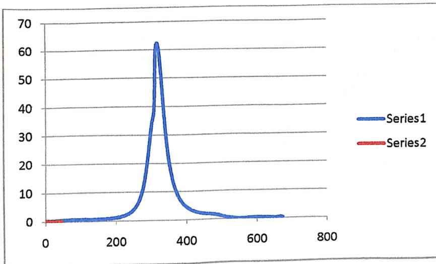
**Crank angle vs heat release**
