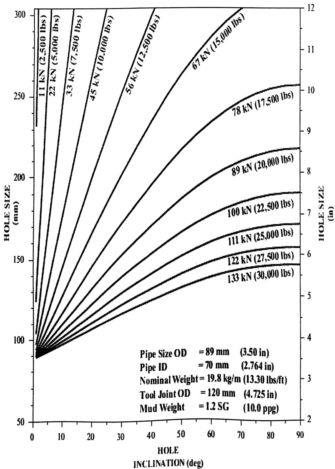
(HELICAL POST BUCKLING LOAD FOR 3-1/2" DRILLPIPE - STEEL 13.30 LBS/FT)
