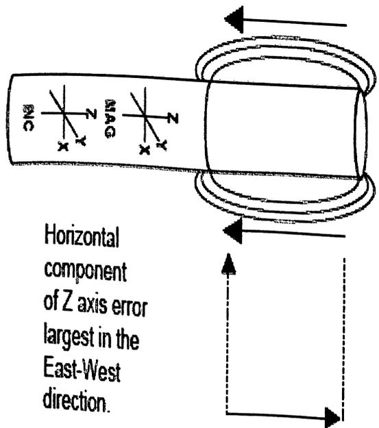
(EFFECT OF AZIMUTH ON DRILLSTRING MAGNETIC INTERFERENCE)
