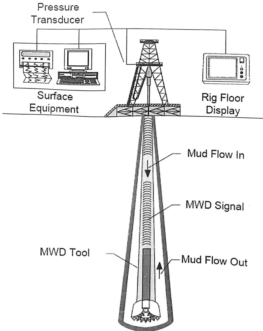
**Figure 4-33 Mud pulse telemetry**
