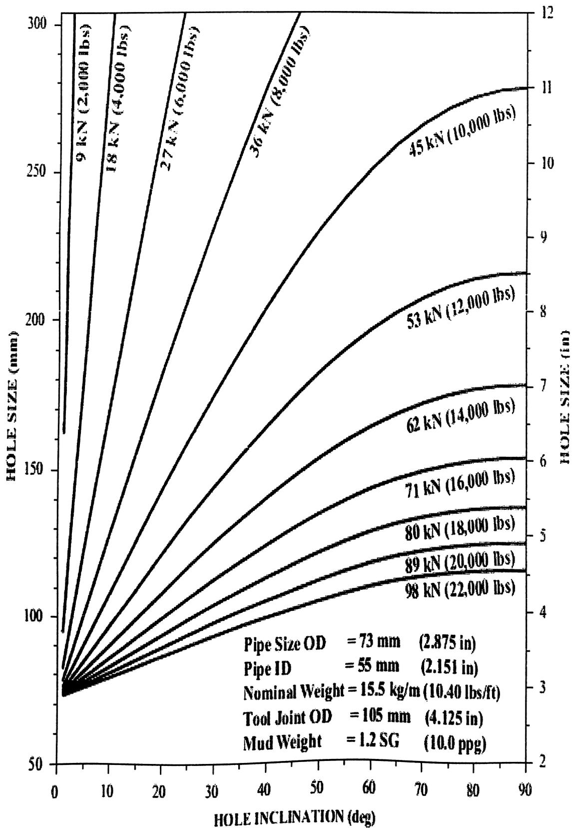
(HELICAL POST BUCKLING LOAD FOR 2-7/8" DRILLPIPE - STEEL 10.40 LBS/FT)
