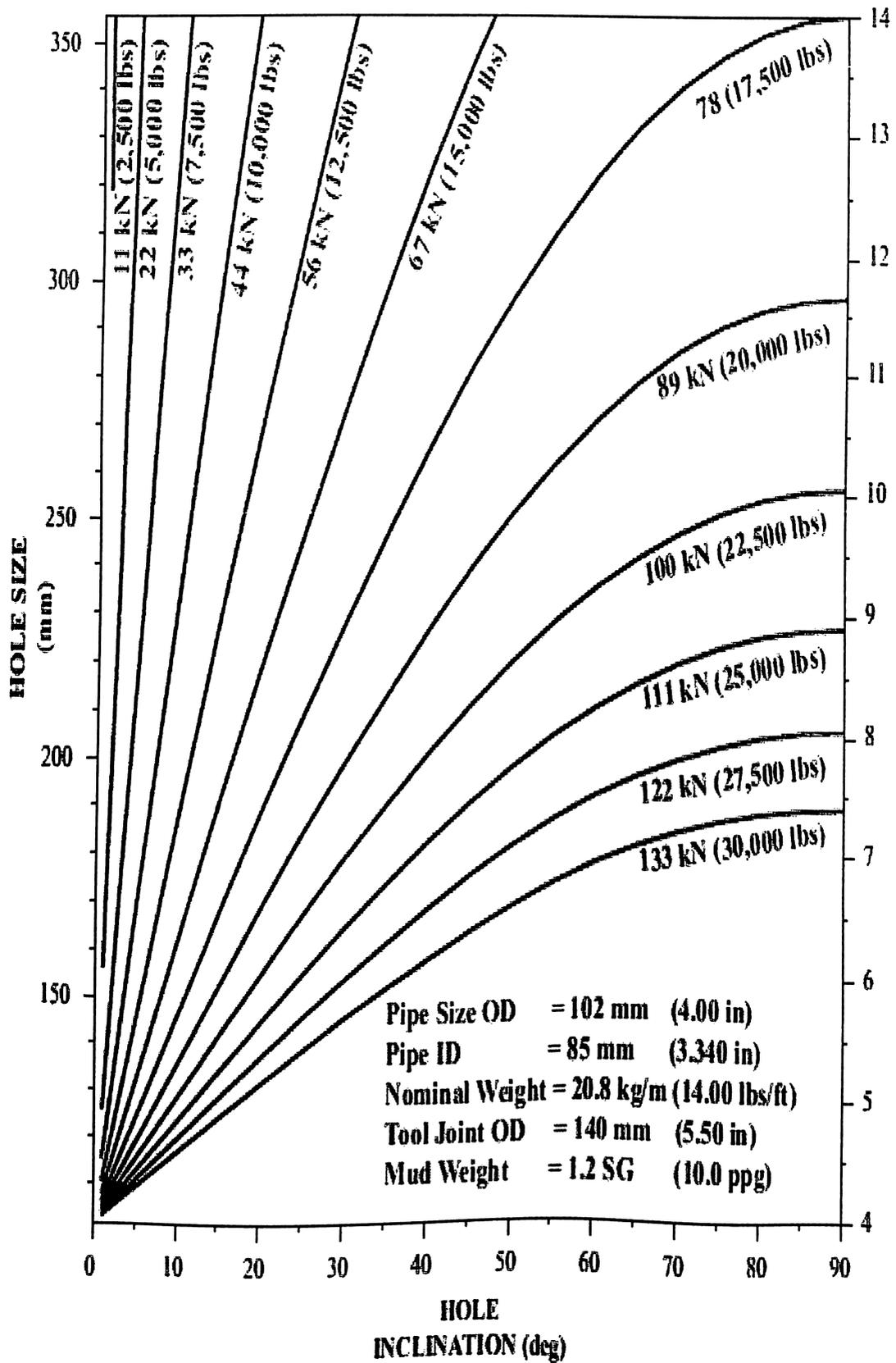
(HELICAL POST BUCKLING LOAD FOR 4" DRILLPIPE - STEEL 14.00 LBS/FT)
