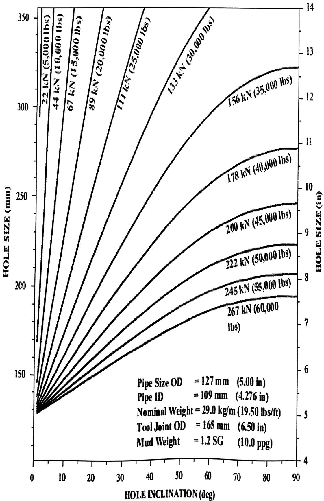
(HELICAL POST BUCKLING LOAD FOR 5" DRILLPIPE - STEEL 19.50 LBS/FT)
