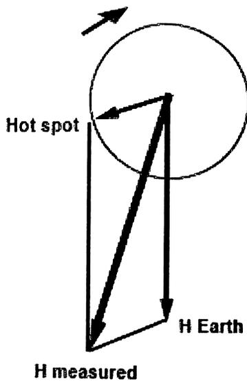
All 3 axis measurements are affected. Fluctuation in total field is observed when MWD tool is rotated. Calculated azimuth will be wrong but will be repeatable with the same tool face.
