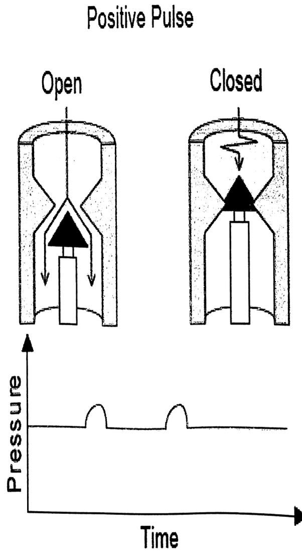
**Figure 4-35** Positive pulse telemetry
