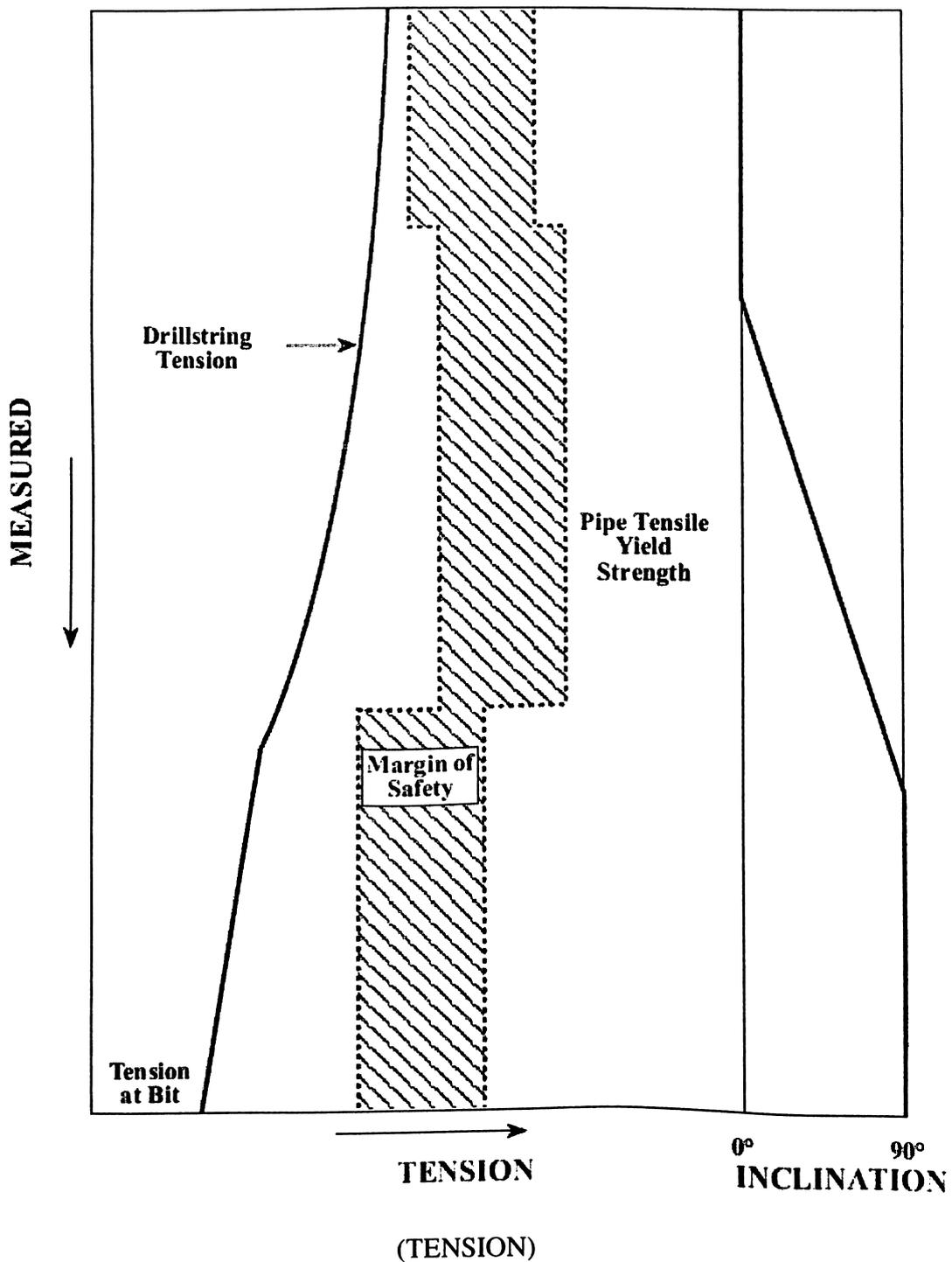
**Tension margin.** The calculated total pickup hookload is increased by 100,000 lbs (or 50,000 lbs if modeling stuck pipe with 50,000 lbs tension at the bit). This new value must not exceed the tensile strength for the particular grade and class of pipe used to ensure adequate tension capability. If the adjusted value of hookload exceeds the tensile strength,
