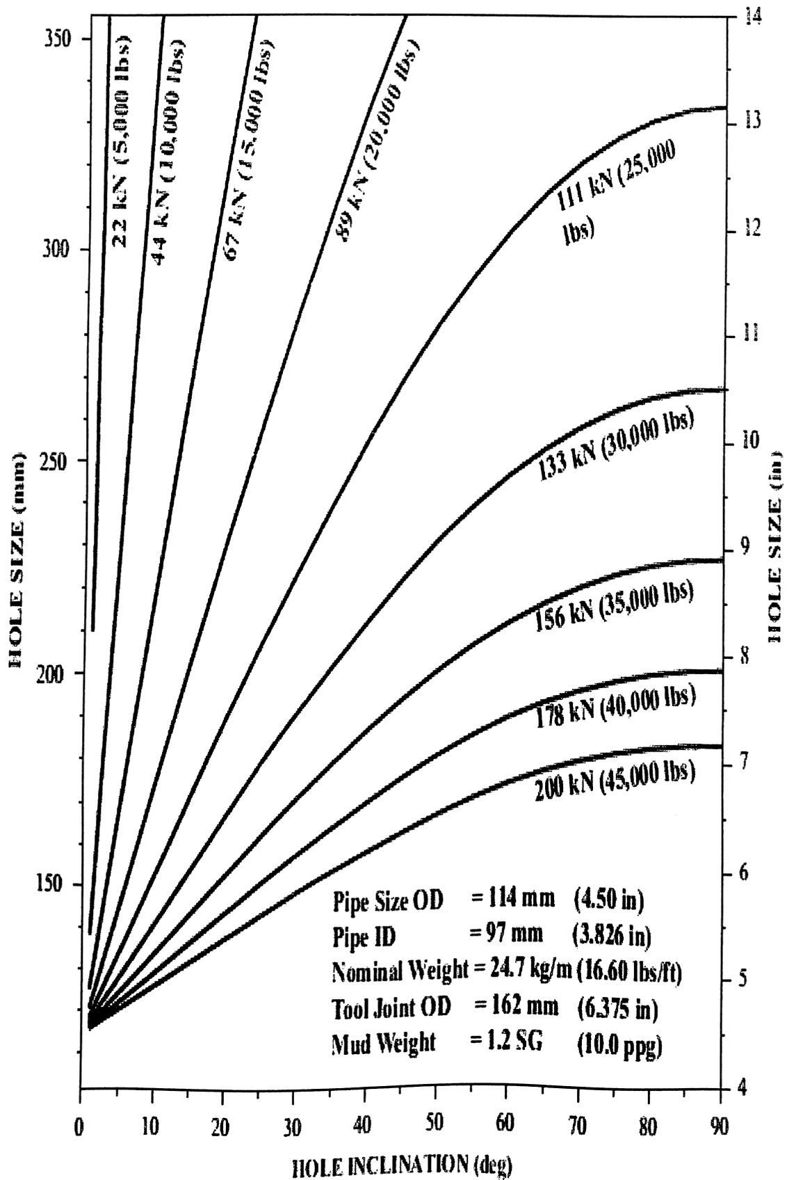
(HELICAL POST BUCKLING LOAD FOR 4-1/2" DRILLPIPE - STEEL 16.60 LBS/FT)
