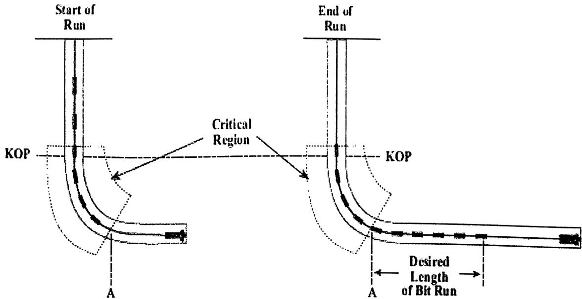
The length of heavyweight must be increased so that heavyweight drillpipe is at point A at the beginning of the run, as well as the end. At the end of this run, compressive forces at point A may have increased to the critical buckling force, and drillpipe will buckle. Therefore, heavyweight drillpipe should be used here.
