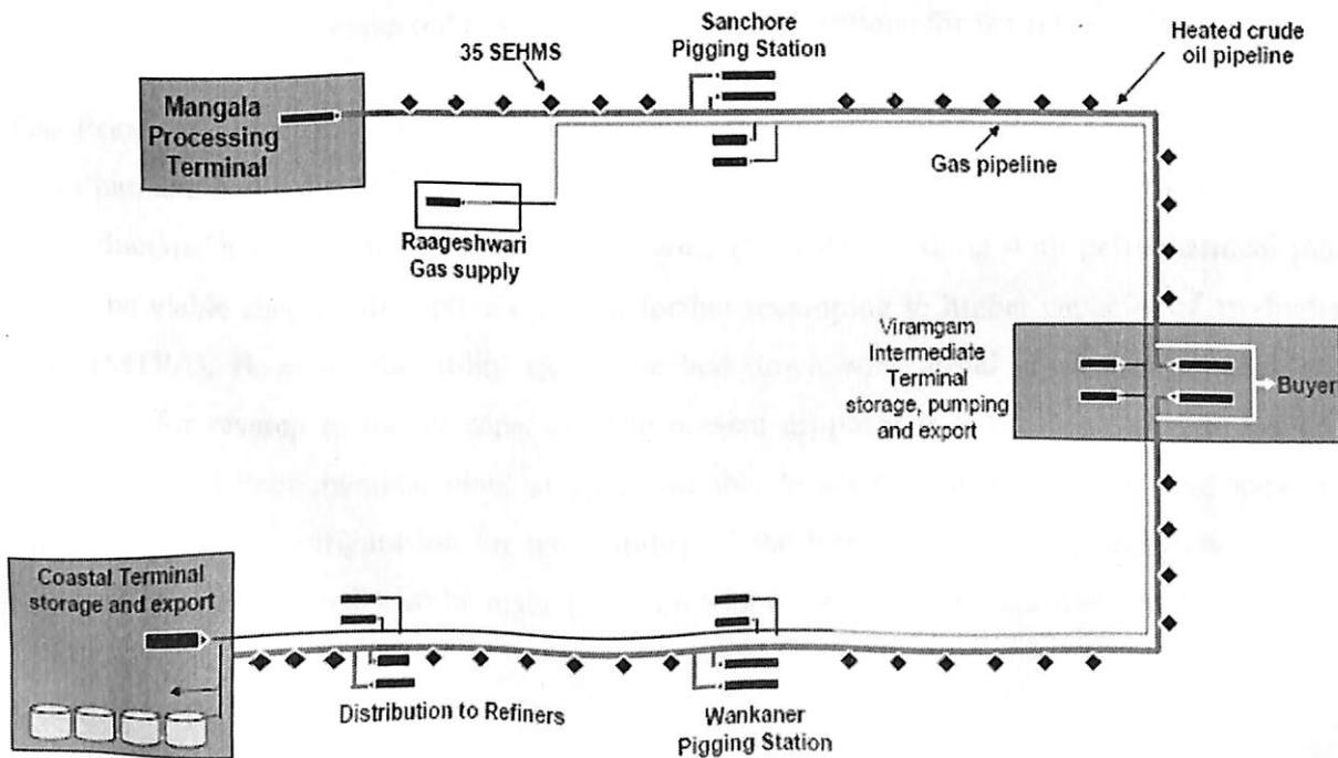
Figure 5: - Pipeline Schematics from MPT to Salaya (Gujarat).
