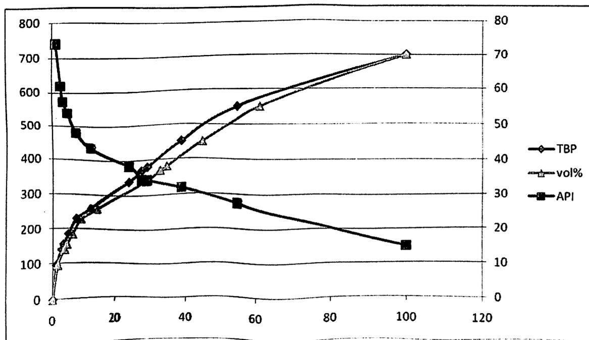
**Figure 6: Extrapolated TBP & API Gravity Curves For Barmer Crude**
