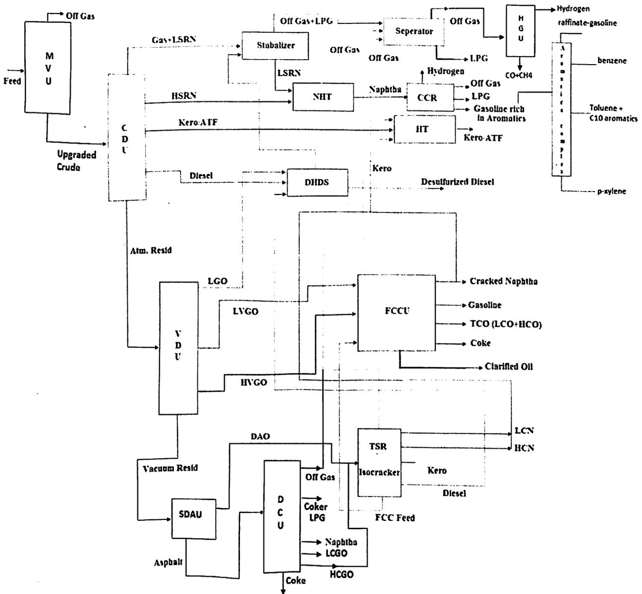
Figure 25: Proposed Barmer Refinery Units Block Diagram with Upgraded Crude
