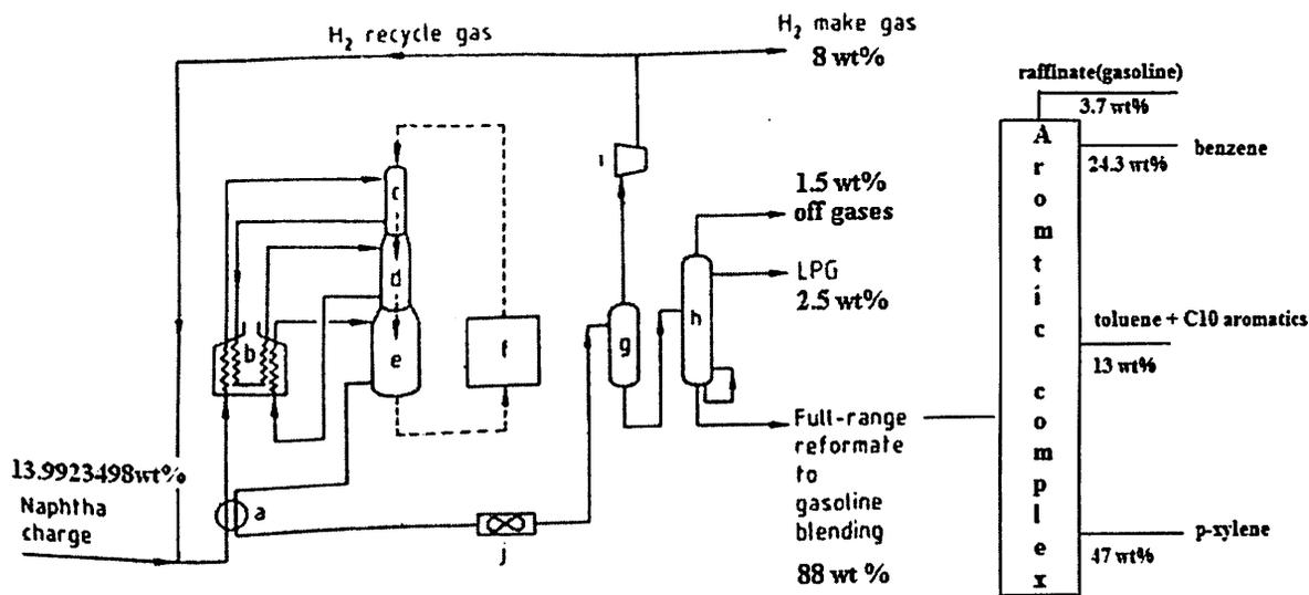
Figure 23: - material balance of CCR and Aromatic complex [19, 20]
