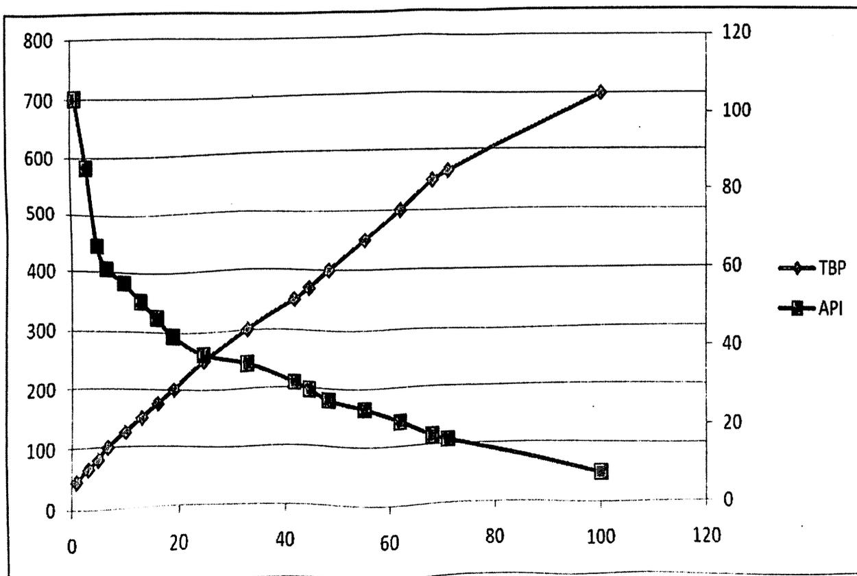
Figure 16: - Extrapolated TBP & API Gravity Curve for Upgraded Barmer Crude
