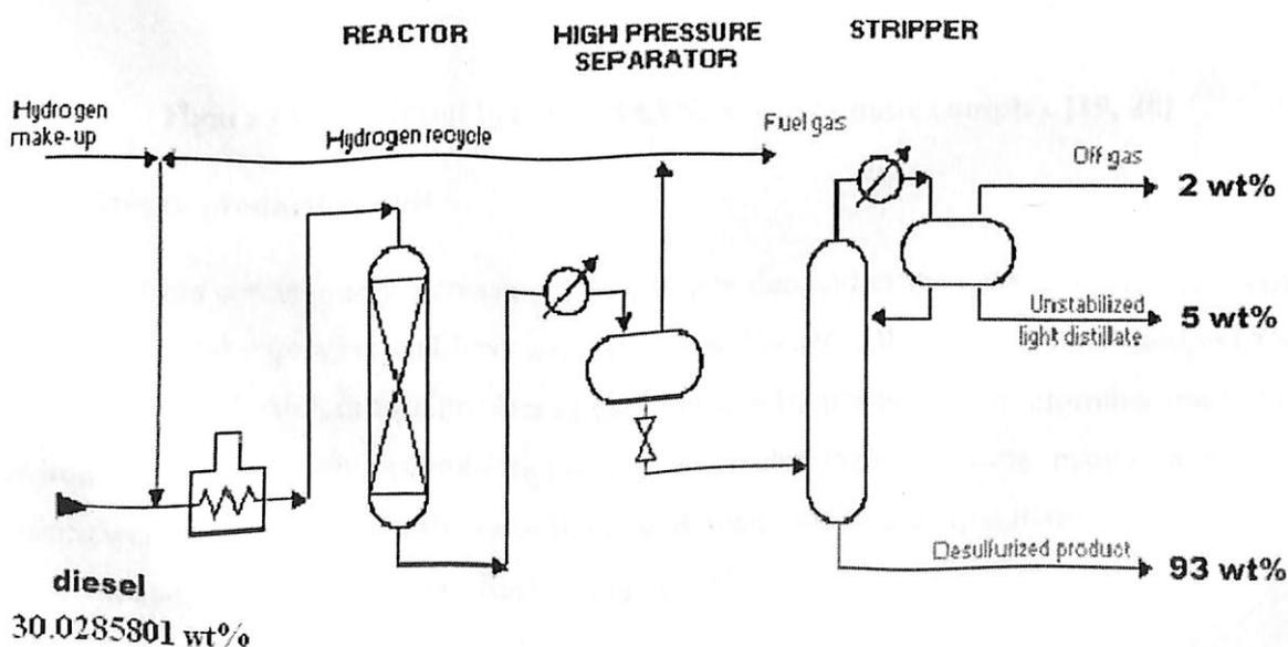
Figure 22: - material balance of DHDS unit in terms of wt%
