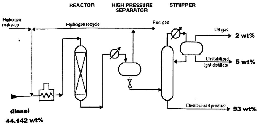
Figure-12-Diesel Hydrodesulfurization Unit
