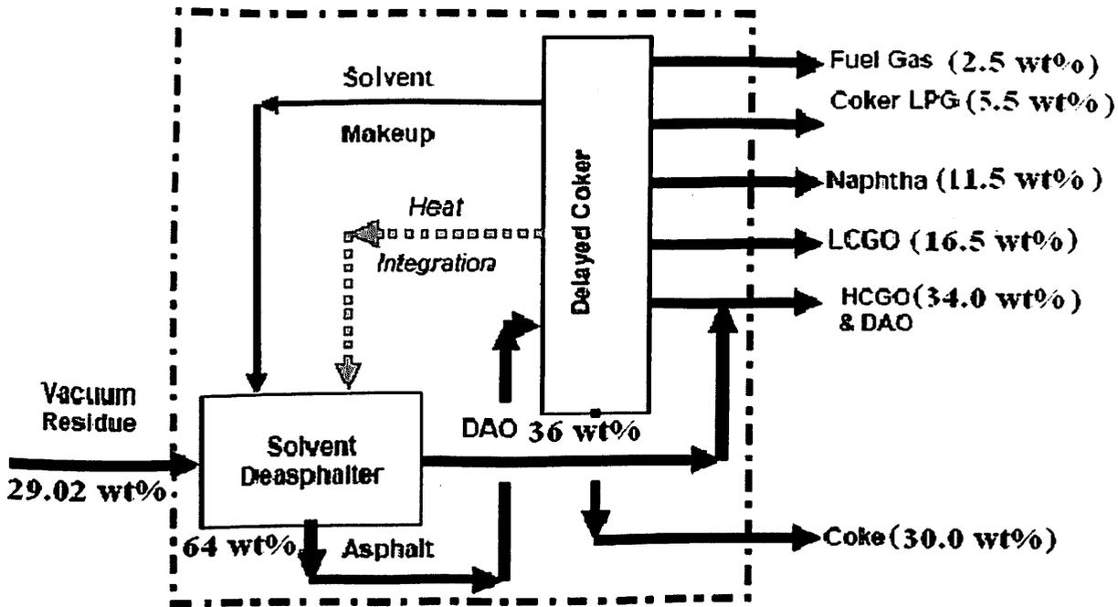
Figure 18: - Schematic diagram of integrated solvent Deasphalting and Delayed coking unit
