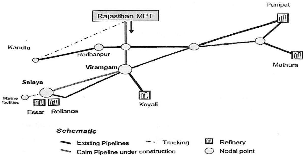
Figure 4: - Existing and upcoming pipelines through Rajasthan
