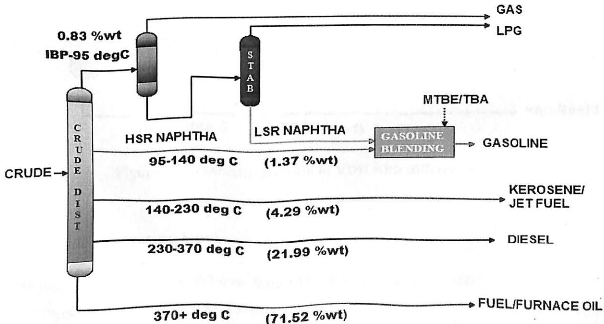
Figure 7: - Schematic diagram of CDU with various cut
