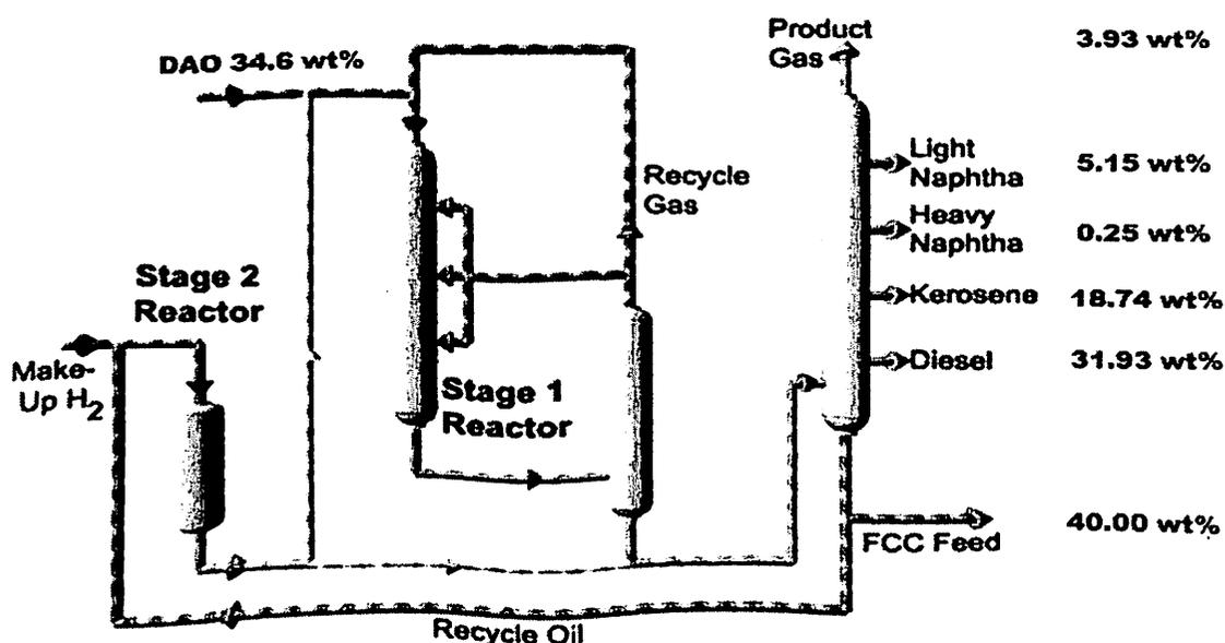
Figure 10- Material balance of Two Stages Recycle Isocracking unit
