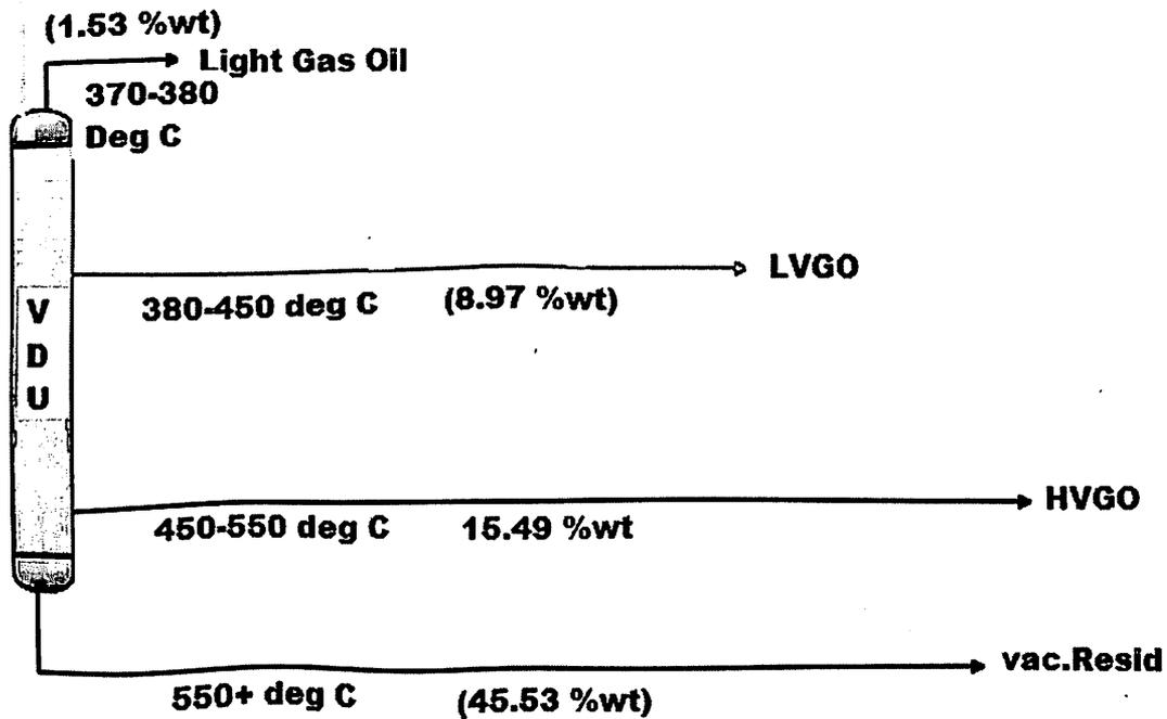
Figure 8:- Schematic diagram of VDU with different cut.
