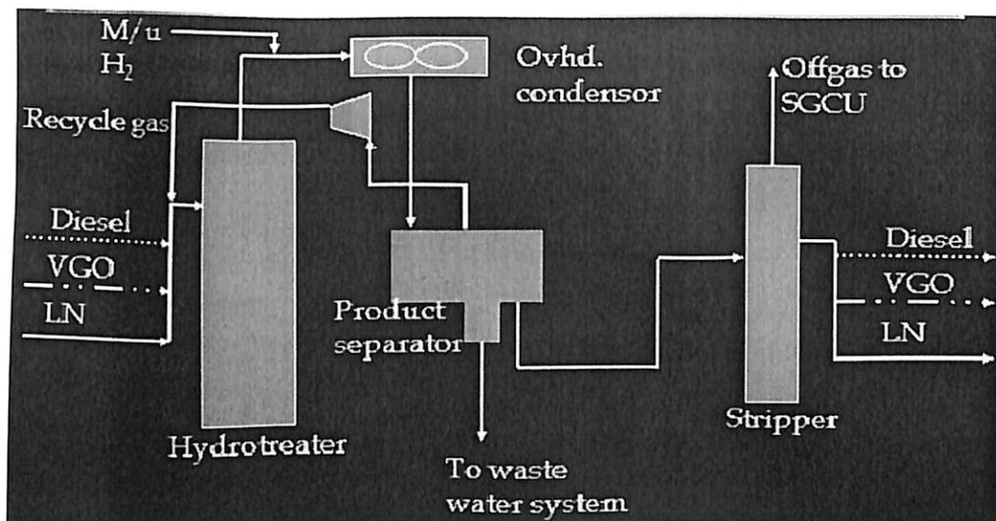
Figure 21: - Schematic diagram of Hydrotreater unit
