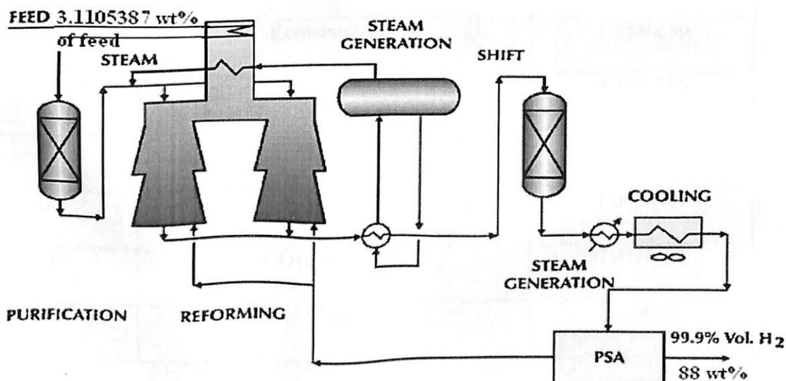
Figure 24: - Material balance for steam methane reforming/PSA
