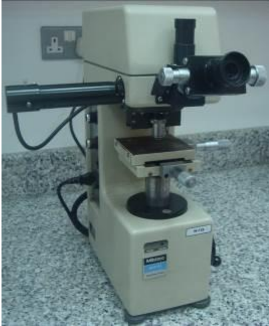
Figure 3.12: Microhardness tester used for hardness measurements
