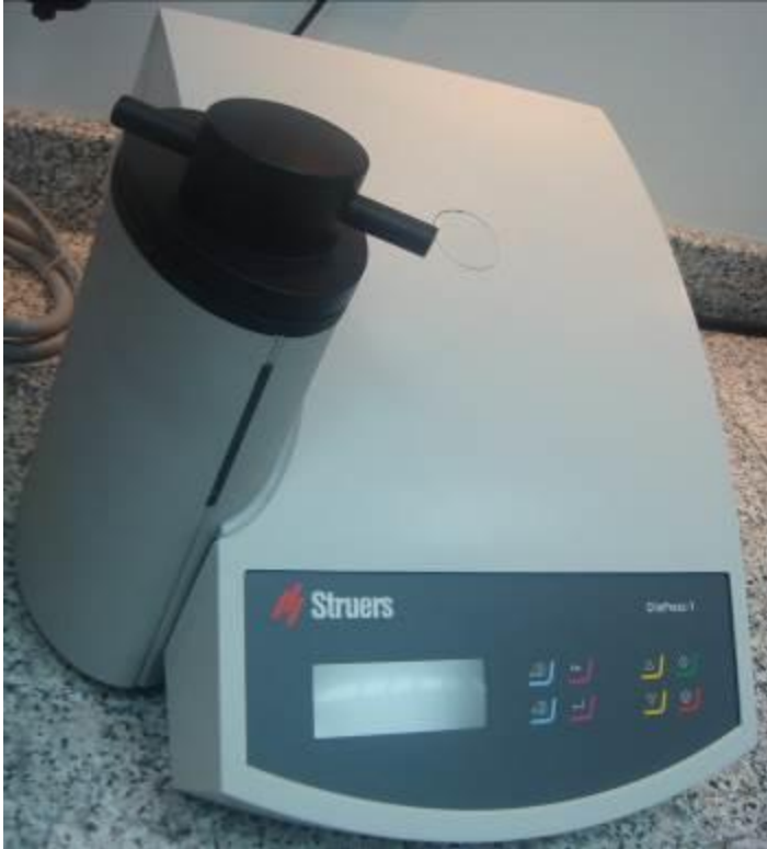
Figure 3.6: The hot mounting press - Citopress
