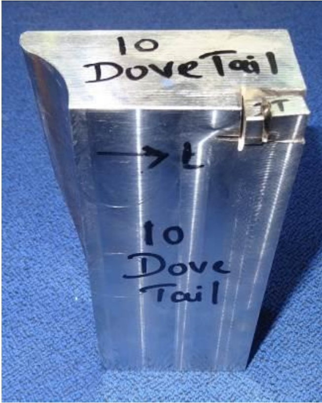
Figure 3.15: Section 10 near the dovetail area after further dissections
