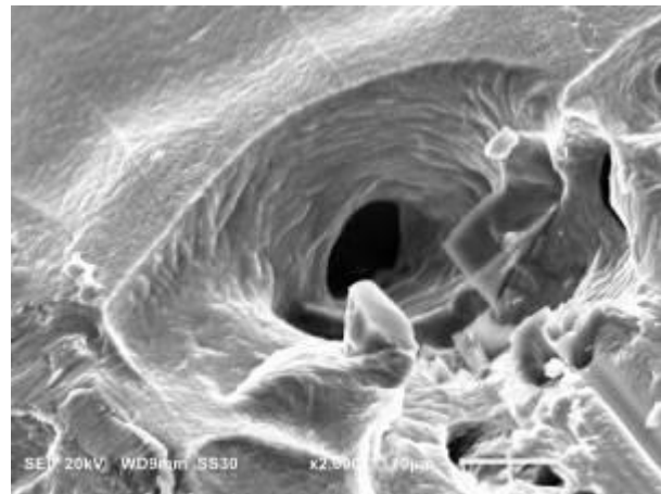
Figure 4.148: SEM micrograph of fractured tensile sample at 21 °C, (SA - 1120 °C x 3 hrs + Age - 600 °C x 8 hrs); Original Magnification - 2000x
