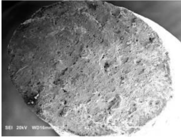
Figure 4.105: SEM micrograph of fractured tensile sample at 450 °C (SA - 950 °C x 3 hrs + Age - 640 °C x 4 hrs); Original Magnification - 33x
