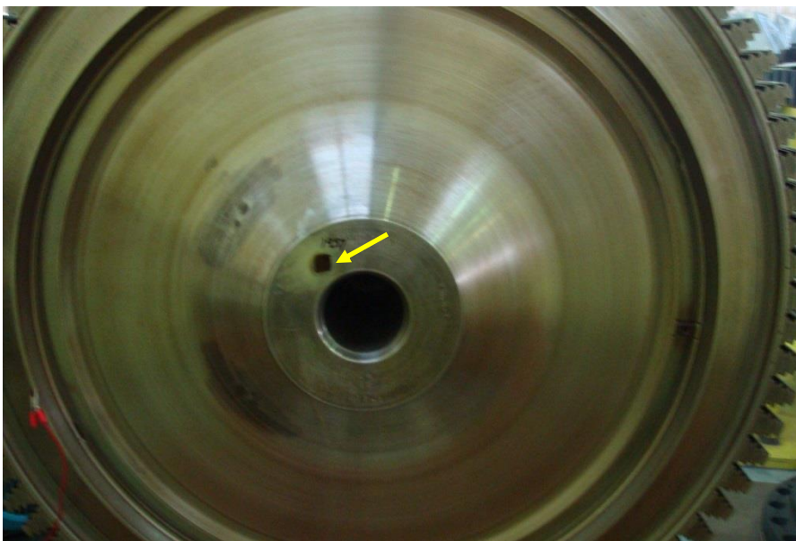
Figure 5.2: Replication Location at the Bore area shown by arrow
