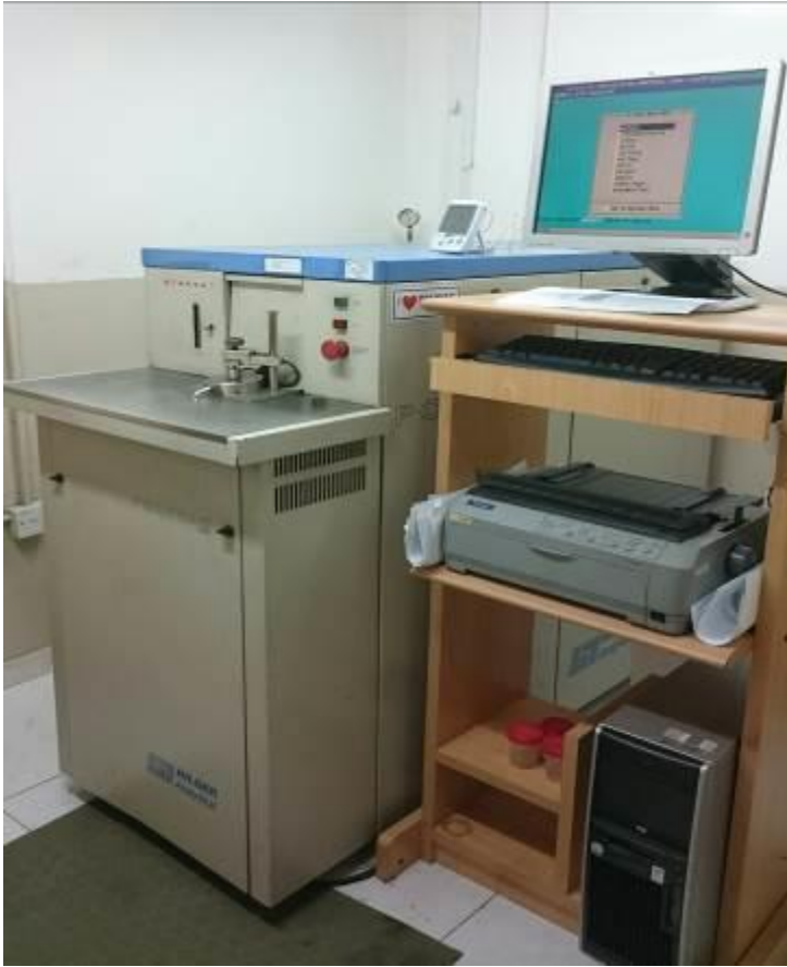
Figure 3.1: Optical emission spectrometer used for chemical analysis
