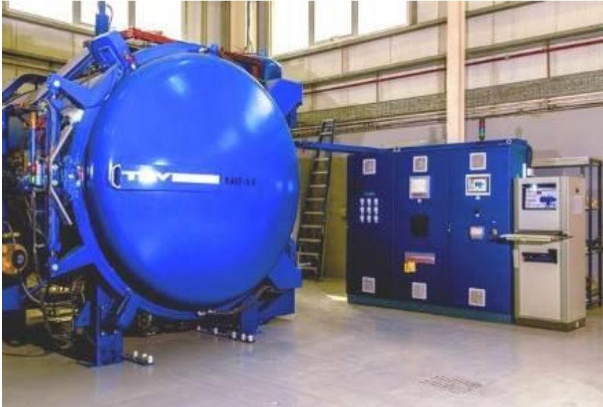
Figure 3.16 – Vacuum furnace used for heat treatments
