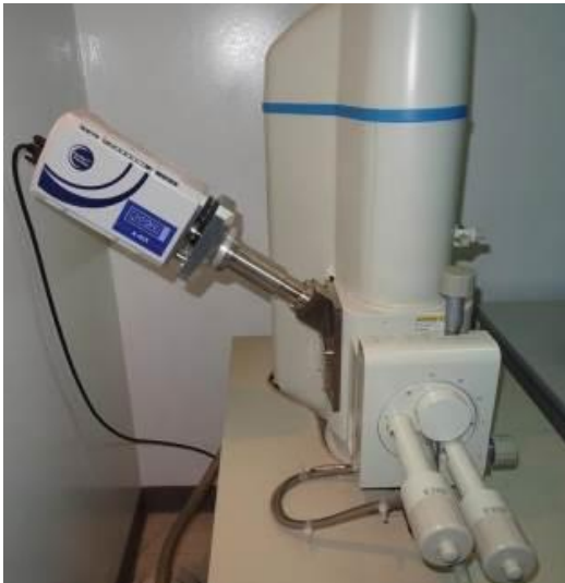
Figure 3.11 – EDAX Detector on the SEM
