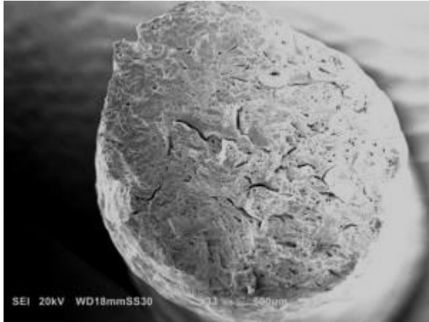
Figure 4.145: SEM micrograph of fractured tensile sample at 21 °C, (SA - 1120 °C x 3 hrs + Age - 600 °C x 8 hrs); Original Magnification - 33x
