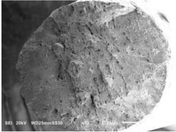
Figure 4.205: SEM micrograph of fractured tensile sample at 450 °C, (SA - 950 °C x 3 hrs + Age - 640 °C x 12 hrs); Original Magnification - 33x
