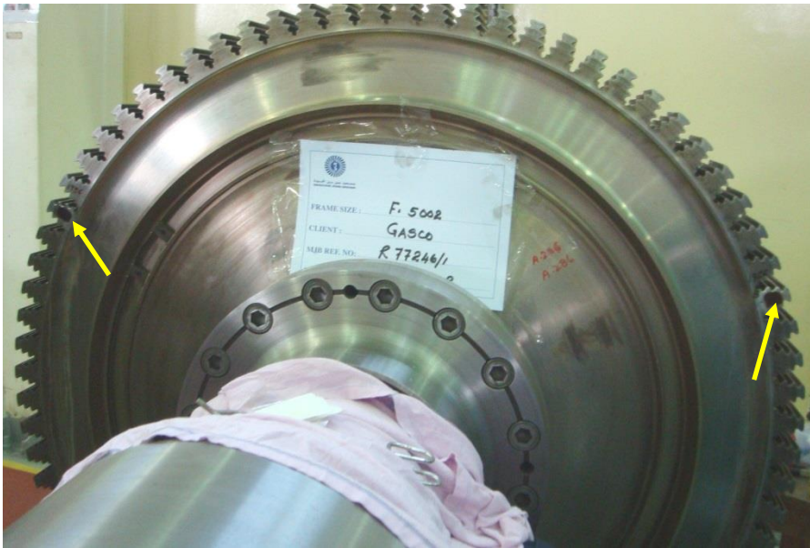
Figure 5.1: Replication Locations at Dove Tail areas shown by arrows
