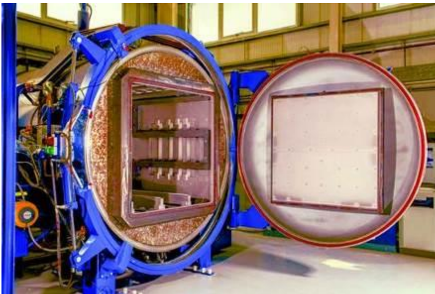
Figure 3.17 – Vacuum furnace showing the internal chamber
