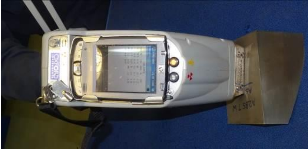
Figure 3.3: XRF analysis on a serviced turbine wheel section
