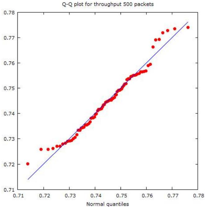
Figure 7-13Q-Q Plot for OSA throughput (500 Packets)
