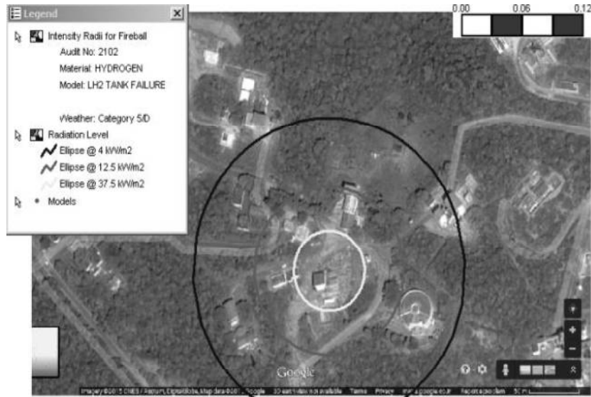
Figure 4.9. Radiation intensity contour for catastrophic failure
