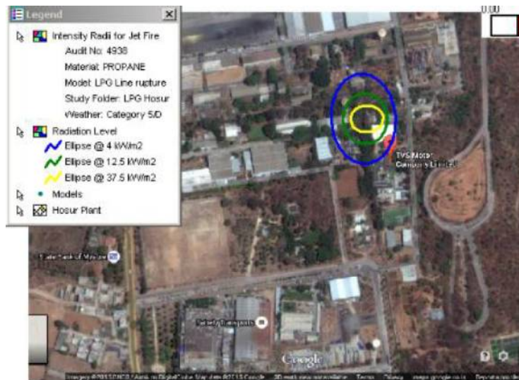
Figure.4.5: Radiation Intensity Contour for Jet Fire
