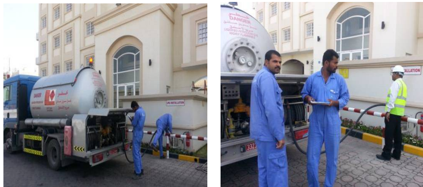
Figure.4.11 LPG gas unloading operation of the apartment
