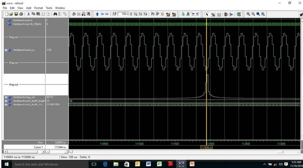
Fig. 6.7.1(c) Simulation result with index ‘11’ and peak starting at 111.944  $\mu$ s when delay=0.41  $\mu$ s
