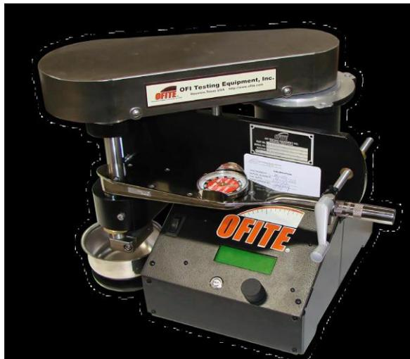
**Figure 24 - lubricity/ film strength tester**
