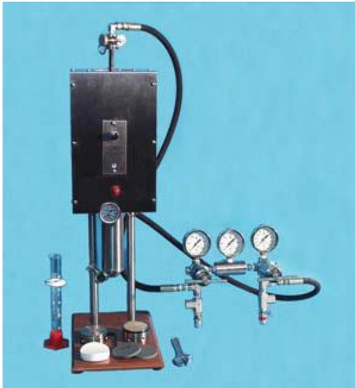
**Figure 22 - HTHP filtration test**
