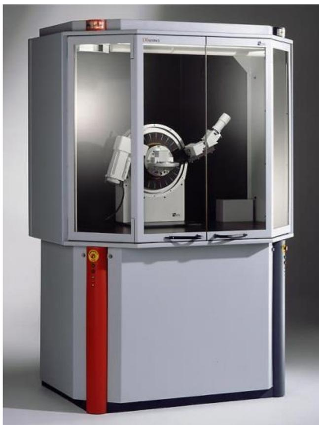
**Figure: 3. 7:** Photograph of Bruker D8 advance X-ray Diffractometer
