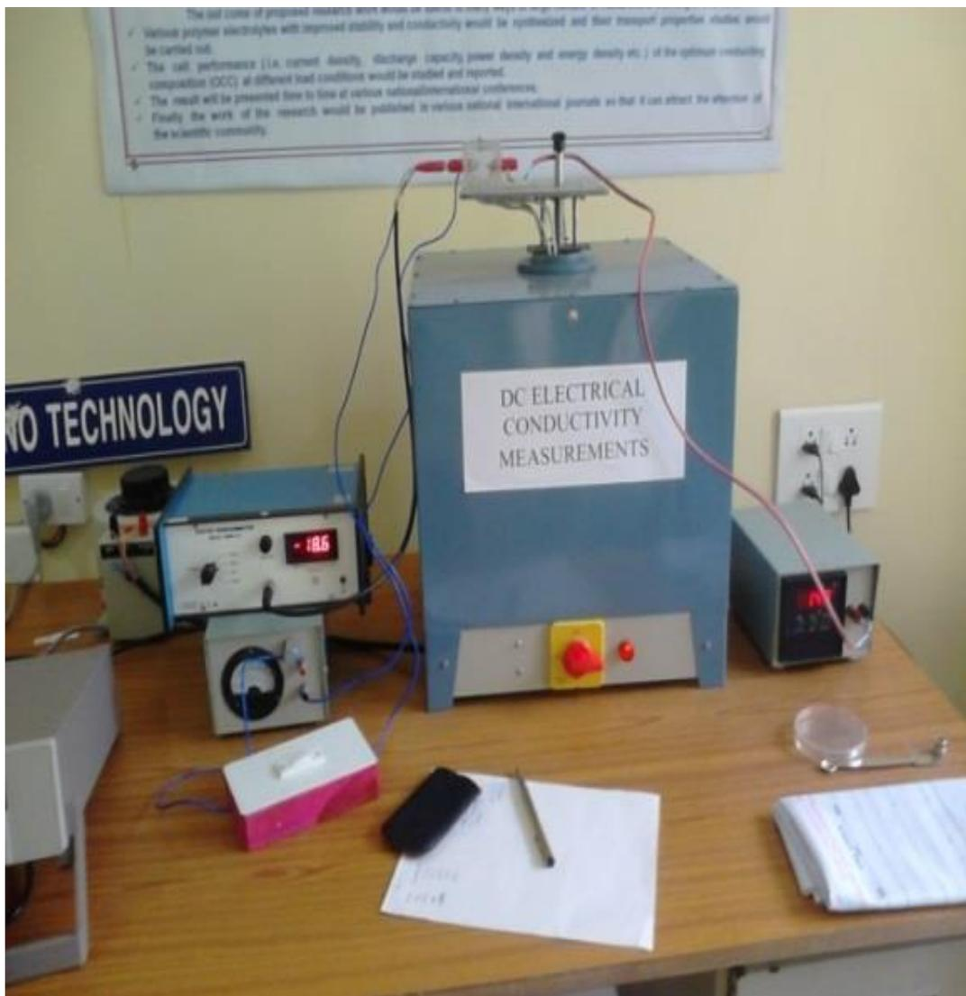
**Figure: 3. 13:** Photograph of dc conductivity measurement setup at KL University, Vijayawada.
